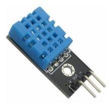
Only three pins are available: VCC, GND, and DATA. The communication process begins with the DATA line sending start signals to DHT11, and DHT11 receives the signals and returns an answer signal. Then the host receives the answer signal and begins to receive 40-bit humiture data (8-bit humidity integer + 8-bit humidity decimal + 8-bit temperature integer + 8-bit temperature decimal + 8-bit checksum). For more information, please refer to DHT11 datasheet.
